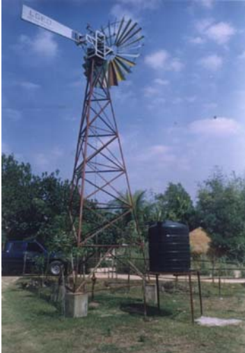
Water Pumping Windmill, designed by LGED
